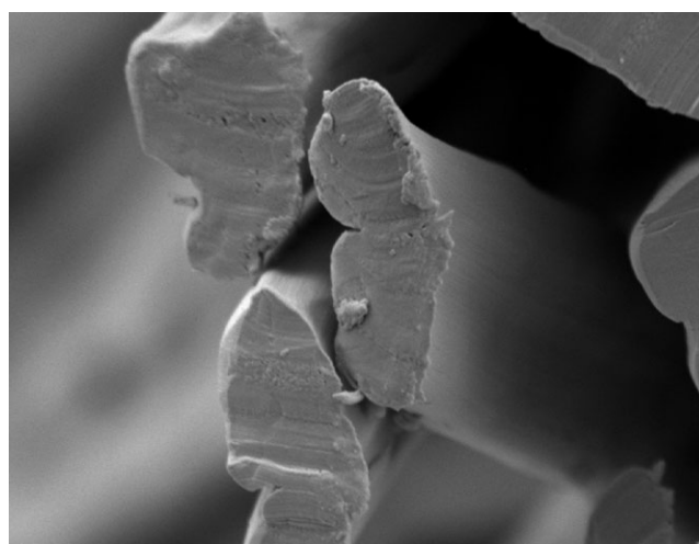
Figure 9. Scanning electron micrograph of the cross-section of oxidatively bleached soybean fiber treated with 5% Byco C.
